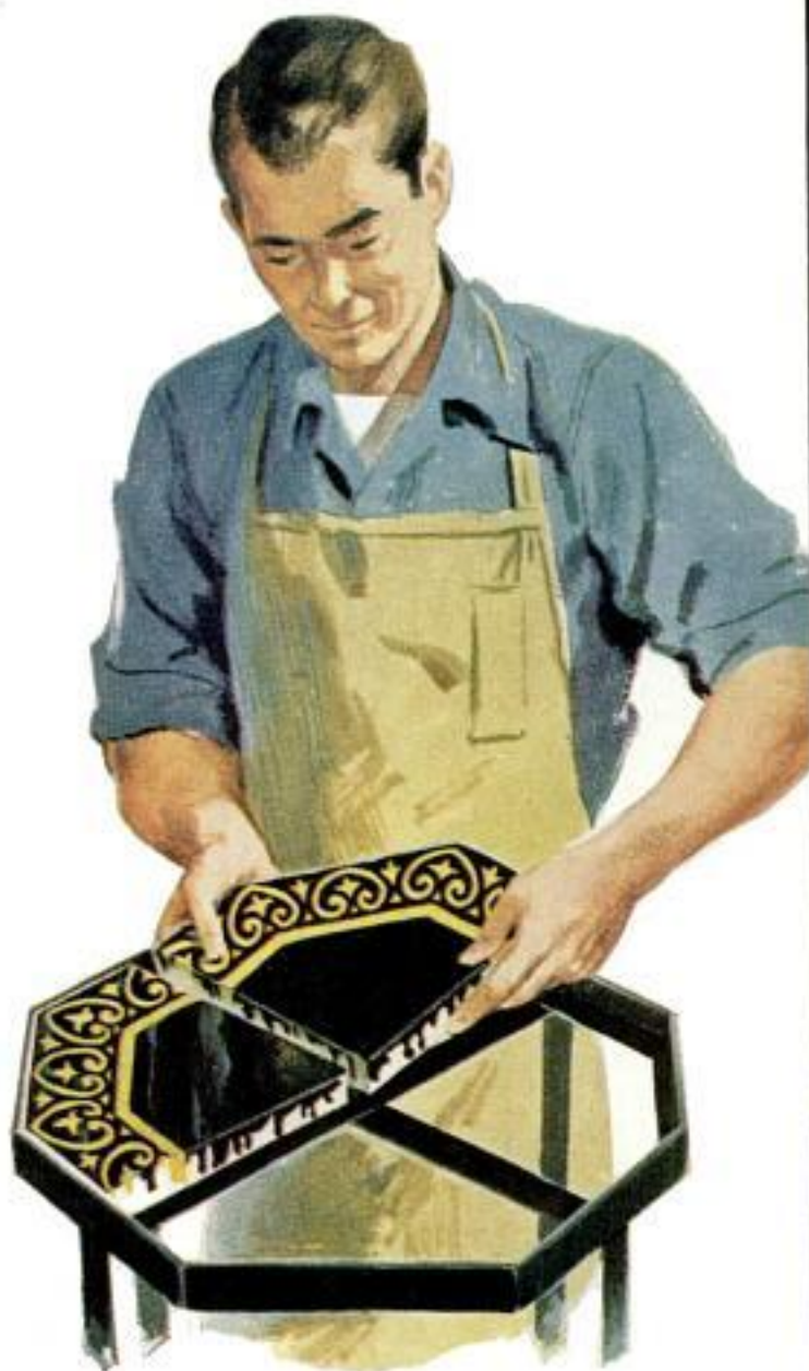
Illustration above shows tile being checked for proper clearance in steel-angle table frame. Hexagonal frame and base were made as in the detail below
